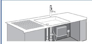
The lonizer is installed under the sink and easy to handle via display which is integrated in the water dispenser.
